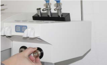
Screwing in the adapter
